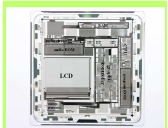
Fig 1- Glass substrate on which system panel of LCDs is formed
